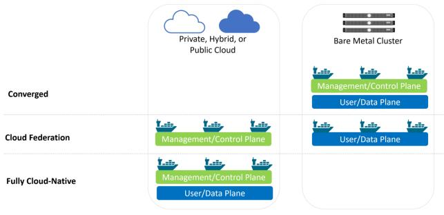
Figure 2 – Entra vCMTS Deployment Models
